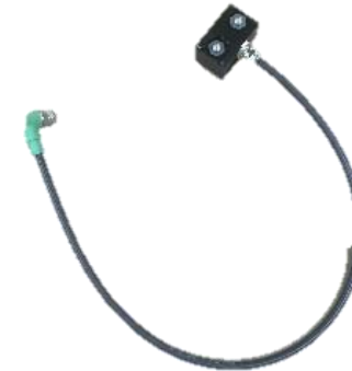
Camber angle measurement via inclinometer
