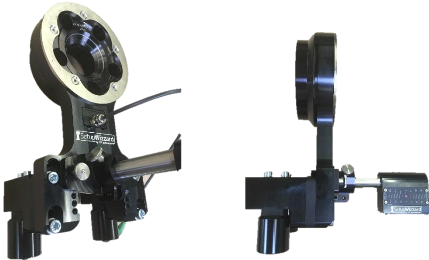
Setup Wheels incl. vehicle specific wheel adapters and stands
