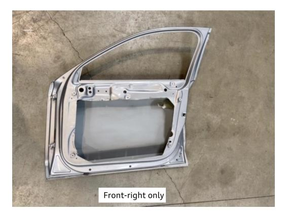
Mark the cut-out with the pattern. Before cutting check the contour by mounting the inner door-cover to. Correct it according to the cover !
