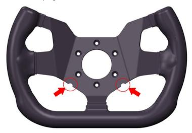
Bushings Ø7.8 x 13mm. Two of the four bushings have to be cut to the length of 7mm.
