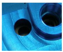
Ensure holes in spools are visually aligned to those in the valve block
