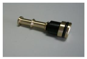
4. Apply **silicone grease** around the o-ring and slide the valve spool over the piston, ensuring that the piston is a good fit, and can cleanly and easily slide within the spool. It is important that the o-ring is greased and if a valve block (or spool assembly) is built and left unused for extended periods (>6months) then they should be re-greased (and re-tested) prior to its first use.
