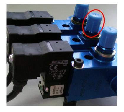
FOR SPECIAL WIRED VERSIONS OF PILOT VALVES, CHECK CORRECT ORIENTATION - SEE BACK OF THIS MANUAL
