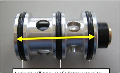
Apply a small amount of silicone grease to the three O-rings on the outside of the spool.
