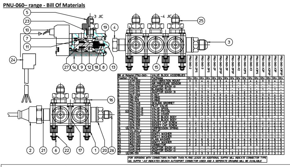
The variations relate to the number of valves within the block (i.e. 2 or 3 valves), if the block has a pressure sensor fitted & what size fittings the outlets have (-3 or -4 JIC).
