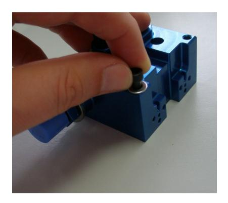
14. Fit AV mounts (AVM-002) to each of the caphead screws and tighten. Loosely fit washers (WSH-069) & k-nuts
