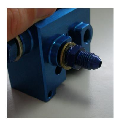
16. Fit either the pressure sensor (ELC-050/075##) or blanking plug (HYD-031) along with dowty washer (WSH-065) ensuring the washer is fully clamped upon tightening.
