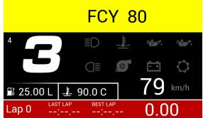
If the car speed is higher than the target limiter speed, check the tyre circumference selected on the ECU clx file (2100 mm as default) that should match with the size of the tyres used on the car.
