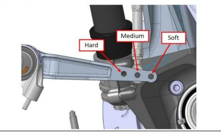
In addition, the drop link can be fixed to the upright in two different positions (ARU) that will change the ARB lever motion ratio and consequently the ARB stiffness.
