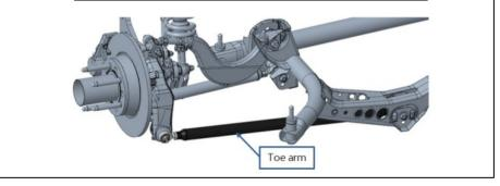
No additional parts are required for setup the rear Camber and Toe. You can achieve the desired configuration using the adjustment rods available on the car.
