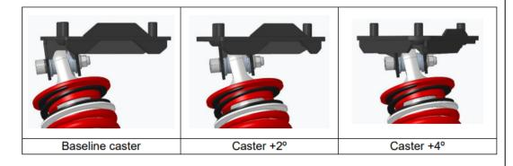
This adjustment will affect to the bumpsteer and it needs to be compensated replacing the steering arm bushings.
