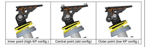
To cover the whole range of camber setting there are three different positions on the top mount and the standard is the central one.
