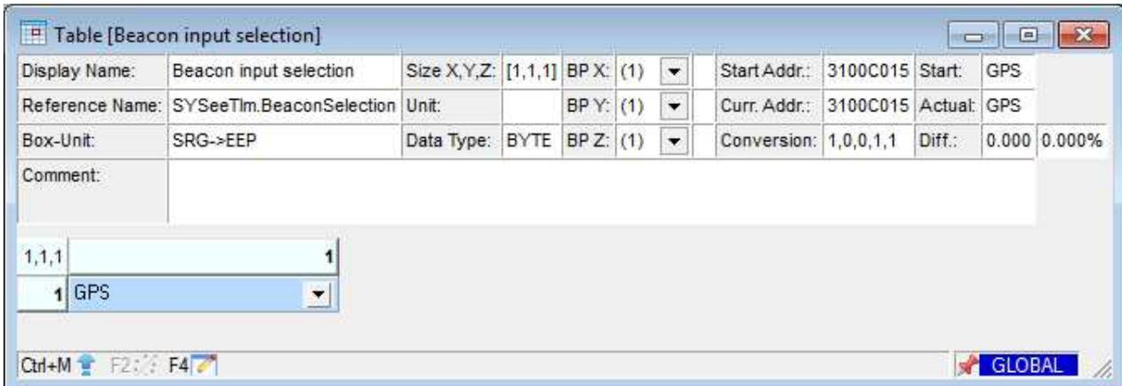
With this calibration set to “GPS”, the logged data will be cut each time the car will cross the virtual track line defined by the GPS POI contained in your SRG 141 TCR (how to set up the GPS POI is described hereafter).
