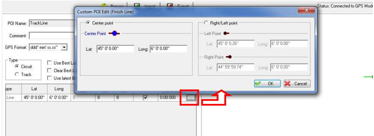
Here, it is possible to change the position of a POI by modifying the coordinates of the central node or also by modifying the positions of the right and left nodes. If the positions of the right and left node are entered, the center node will be automatically calculated.
